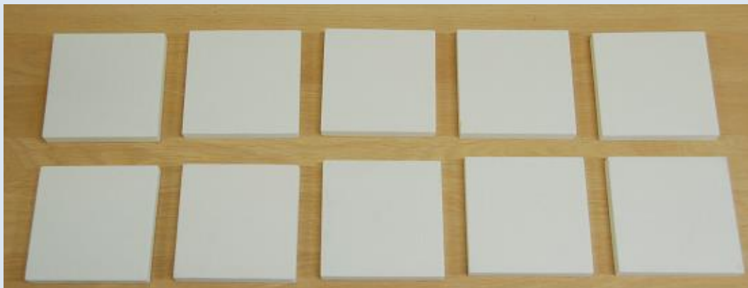
Figure 4.1 – Solid surface 80mm x 80mm samples
